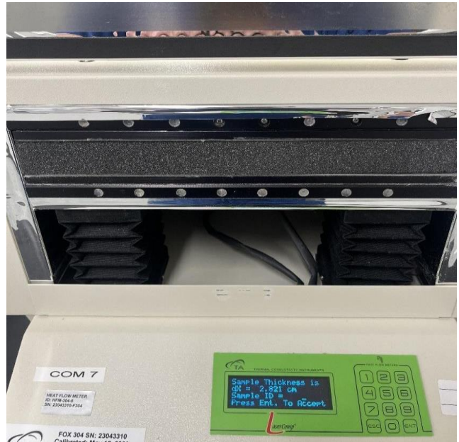
Figure 2. Test specimen in the heat flow meter apparatus
